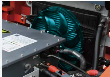
Standard High-Efficiency Liquid Cooling System: Meets automotive S1 duty cycle requirements for continuous operation.
