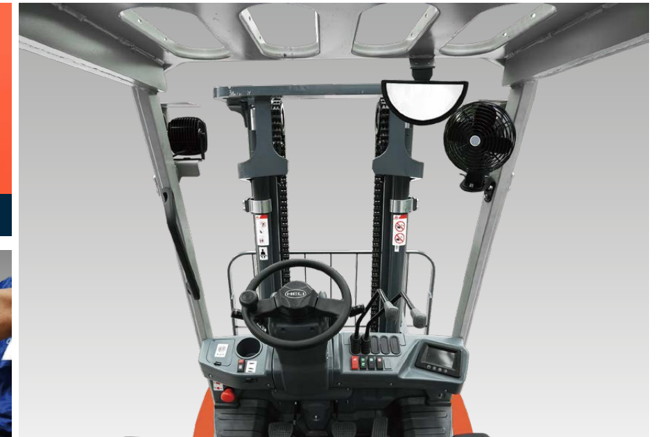
Wide-view Mast: Optimized design minimizes blind spots for safer and more comfortable operation.
